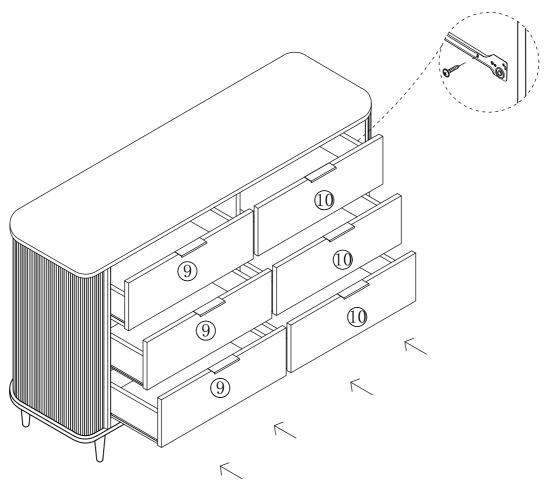
Align the drawer parallel with the slide slots on both sides and slowly push it inward.
