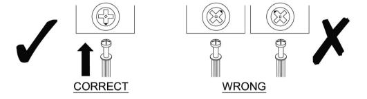
When fitting the cam lock, ensure the starting position is correct before you insert the connecting quickfit.
