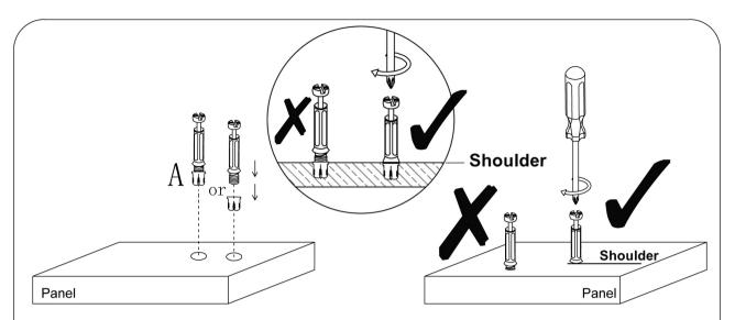
Tighten quickfit until shoulder is flush with the panel. Do not overtighten or undertighten.
